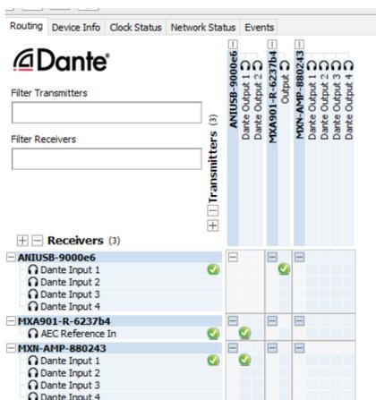
3. Send audio from the ANIUSB-MATRIX to other sources using the ANIUSB-MATRIX's matrix mixer. Open the ANIUSB-MATRIX web application with Shure Update Utility. A common destination is a computer connected by USB with video-conferencing software (such as Zoom or Microsoft Teams).
