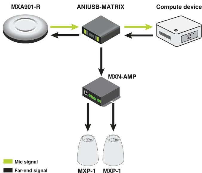
2. Open the videoconferencing software on the computer connected to the ANIUSB-MATRIX. In the settings, choose ANIUSB-MATRIX as the speaker and microphone.
