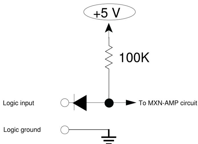
**Important:** Make all logic ground connections to the ground pin, including power supply ground of external logic circuitry. To avoid switch clicks, do not connect logic ground to audio, chassis, or rack grounds.
