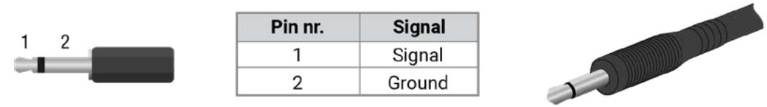
Microphone audio plug pin assignments
